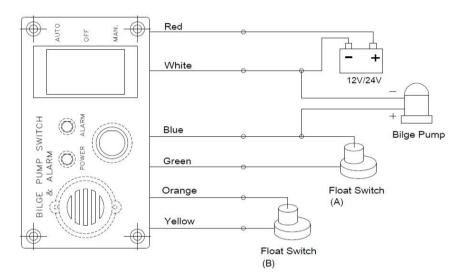
Use min #16 gauge marine grade electrical wire.
